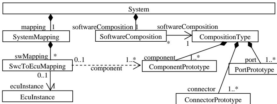
Fig. 3. The AUTOSAR System Template containing relevant types used by our transformation.
