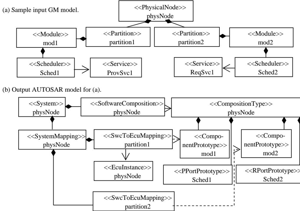
Fig. 4. (a) Sample GM input model and (b) its corresponding AUTOSAR output model.
