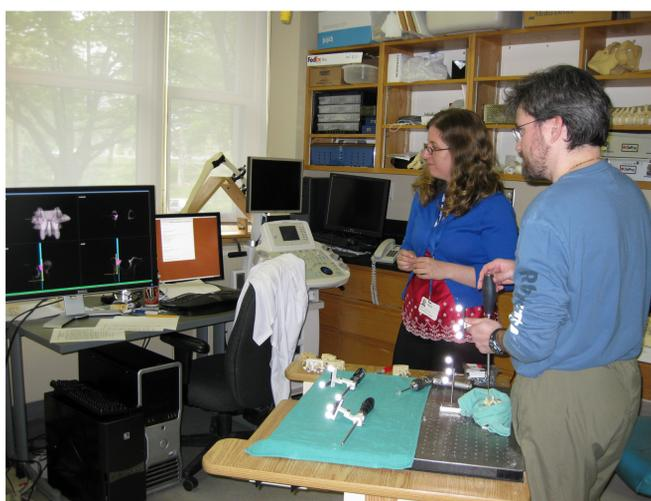
**Figure 4:** Experiment setup used in navigation study. The subject was using the navigation system to guide a tool. The optical tracking system was located just out of the camera frame, to the left.
