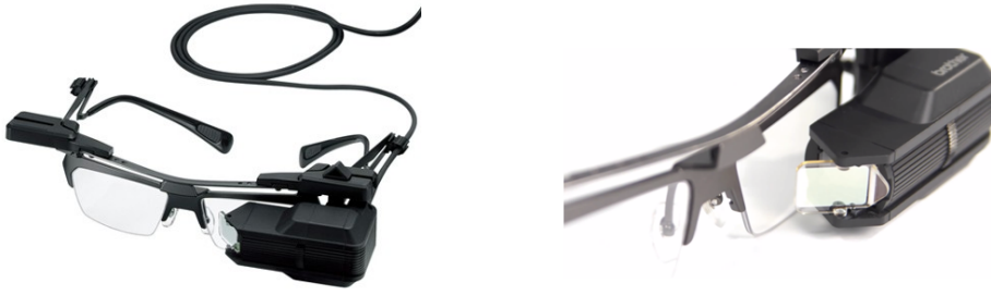
Fig. 3 The Brother AirScouter monocular wearable display. The screen could be positioned in front of either eye. We added a bracket on each side (not shown here) to mount the display higher and slightly outside, converting the through-the-lens display in to a peripheral display. (Unfortunately, our equipment was repurposed for another experiment and the brackets lost before we thought to photograph the entire apparatus together. Here we provide stock images from the Brother website, to be replaced by our own photographs in a published version.)
