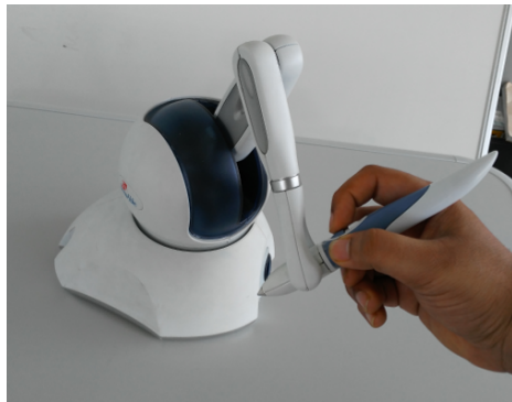
Fig. 2 The Phantom Omni, which served as the tool to be posed on the knee. The experimental subject pressed the button on the pen of the Omni when the pen was deemed to be in the correct pose.
