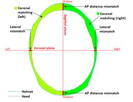
Figure 7. Measures of fit between the helmet and head, as displayed in the Helmet Fit Viewer's viewing panel.
